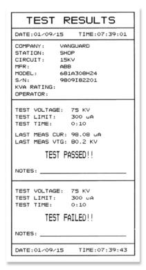
If DC voltage of equal magnitude to the peak of the AC voltage whose magnitude is 75% of the Power Frequency Withstand Voltage Rating of the circuit breaker is applied and withstood for 1 minute, then the vacuum interrupter has an acceptable level of vacuum and is therefore good.
