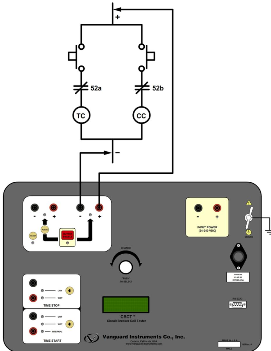
Figure 2. CBCT Constant Output to CB Control Circuits
