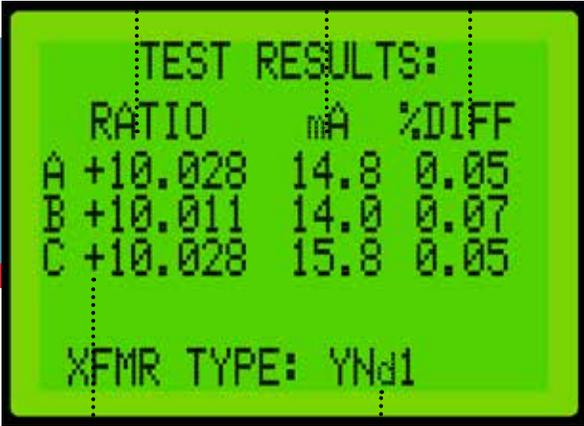
Winding Polarity      Transformer Type
